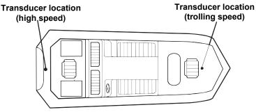
Shoot-thru-hull transducer locations for high speed or trolling speed operation.
